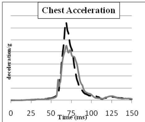
Figure 17. Head and chest Acceleration in US sled test @ 27 km/h with a convertible seat. Dotted lines represent baseline CRS, solid lines illustrate the same CRS with SICT
