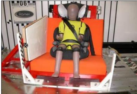
Figure 7. EU internal test method Fixed door on a R44 rig
