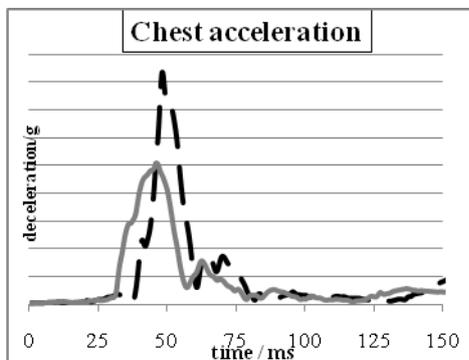
Figure 18. Head and Chest acceleration in EU BIW sled test @ 27 km/h with a booster seat
