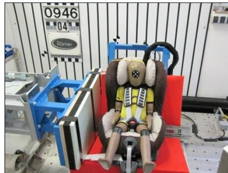
Figure 10. Illustration of EU draft side impact test procedure, moving sled-fixed door
