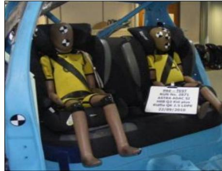
Figure 9. Internal reproduction of the ADAC-Stiftung Warentest side impact BIW test procedure
