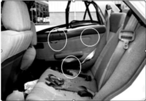
**Figure 20. Examples of vehicle rear seat compartment where energy absorption might be needed for child protection**
