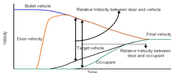
**Figure 6. Physics of side impact – Schematic velocities of bullet car, target car, door and occupant. The parameter to address in CRS domain is the “Relative Velocity between door and occupant”.**
