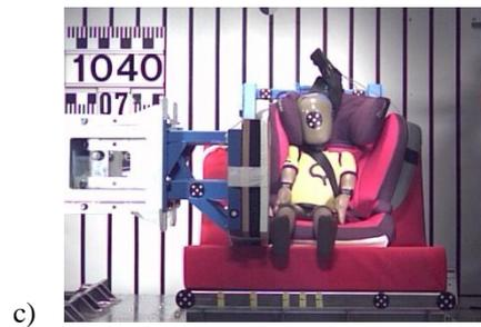
**Figure 16. Principle sequences during a side impact sled test, head is contained through the entire duration of the impact, in a side impact sled test with a Q3 dummy, according to the draft EU side impact test procedure, moving sled-fixed door.**
