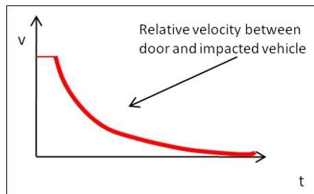
Figure 11. Relative velocity-time relationship of the door in the impacted vehicle. Part of the curve shown in the figure is to be reproduced in the EU draft test procedure.
