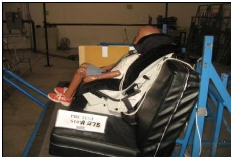
Figure 8. US internal test method Fixed door on a FMVSS 213 rig
