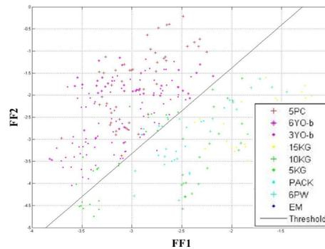
**Figure 10.** Example of discrimination among the most critical occupants from the last test campaign. Three different road styles and vehicle velocities of 50, 70 and 90 kph.
