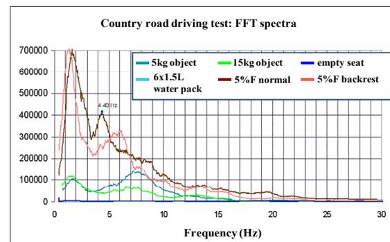
**Figure 5. Frequency spectrum of 5<sup>th</sup> percentile female and of seat cargoes up to 15 kg during 50 km/h cruising on smooth road.**
