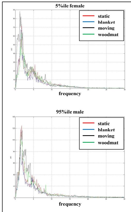
**Figure 11. Seat resonance spectra of 5<sup>th</sup> percentile female (top) and 95<sup>th</sup> percentile male (bottom) sitting on other objects (blanket, wooden mat).**
