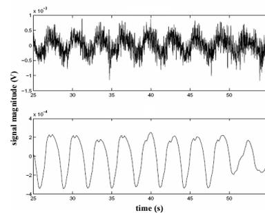
**Figure 1. Vital signals from 50<sup>th</sup>ile male passenger in steady vehicle with engine on: raw signal (upper) and extracted human respiration after wavelet denoising (bottom).**
