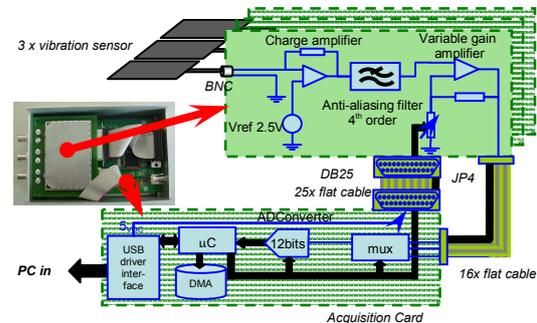
**Figure 9. Block diagram of acquisition electronic interface.**
