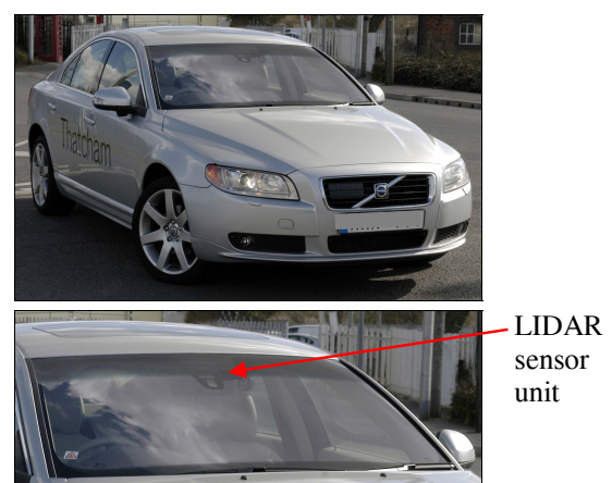
Figure 3. Road driving test vehicle fitted with City Safety.
