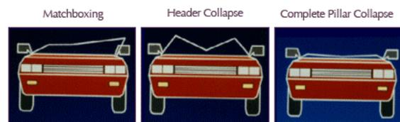
Figure 1. Various Types of Roof Crush
