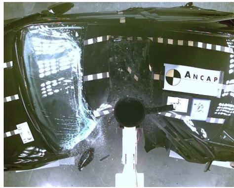
Figure 8. ANCAP research crash test at 50km/h
