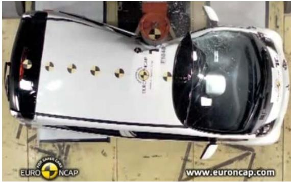
Figure 6. Overhead view at peak of 29km/h pole impact test of an i-MiEV (Euro NCAP)
