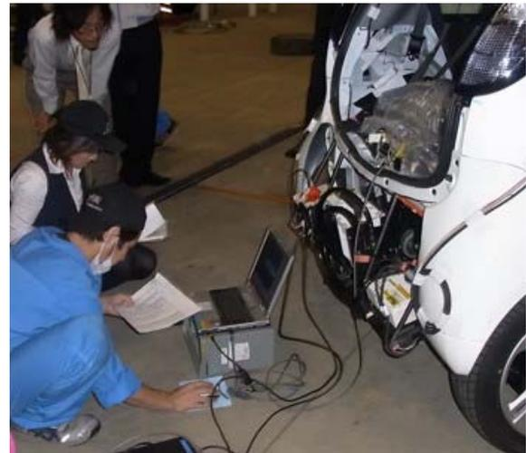
Figure 4. Post-crash electrical tests (ECE 2010)
