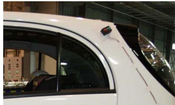
Figure 5. Visual indicator of active high voltage used by JARI during the ANCAP crash test
