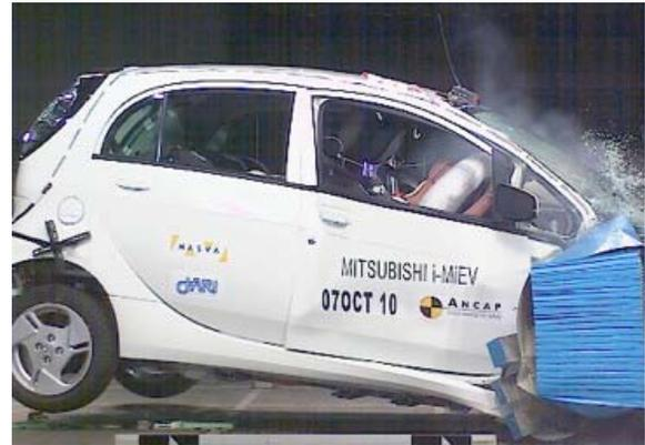
Figure 3. 64km/h offset crash test conducted by JARI for ANCAP
