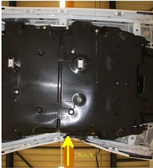
Figure 7. Post-crash underside view of vehicle deformation. Battery pack is under the plastic panel at left (Euro NCAP)
