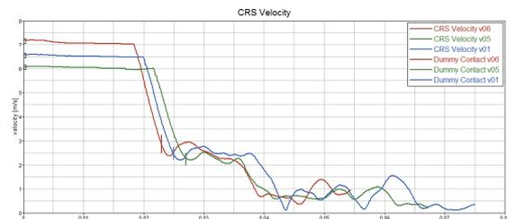
**Figure 29. CRS velocity profiles for the sled delta-v variation.**
