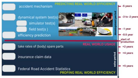
Fig. 2: Continuous evaluation process of real world effectiveness of primary safety measures
