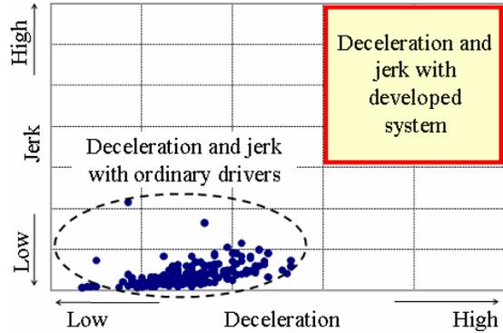
Figure 11. Deceleration and jerk during normal braking by ordinary drivers.
