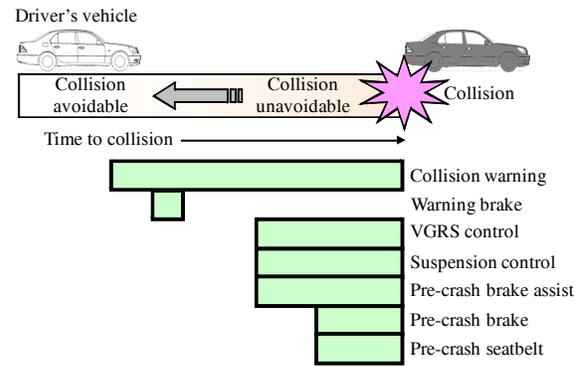
Figure 5. Operation sequence of collision avoidance assist devices.
