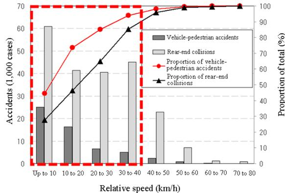
Figure 1. Relative speed distribution of rear-end collisions and vehicle-pedestrian accidents (source: Institute of Traffic Accident Research and Data Analysis (ITARDA) 2010 Report).
