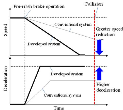
Figure 6. Expansion of automatic braking effect.
