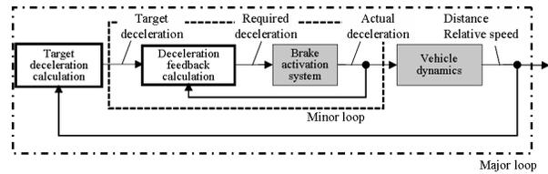
Figure 9. Deceleration feedback control.
