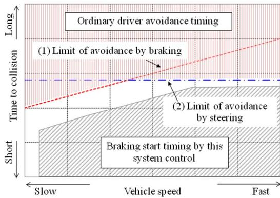
Figure 10. Braking start timing of developed system.
