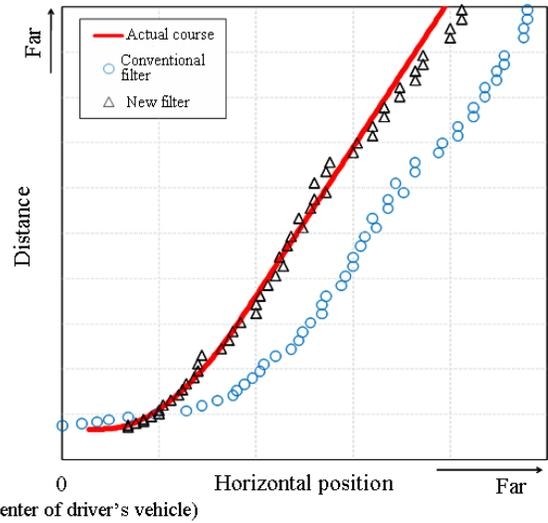
Figure 14. Results of millimeter wave radar horizontal position response comparison (speed of driver's vehicle: 30 km/h, crossing speed of pedestrian: 5 km/h).
