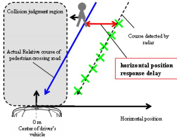
Figure 13. Issue of millimeter radar wave horizontal position response.
