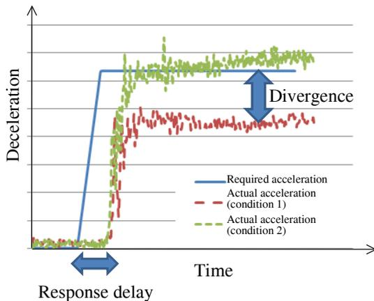
Figure 8. Difference between required and actual deceleration (stationary object, relative speed: 40 km/h).
