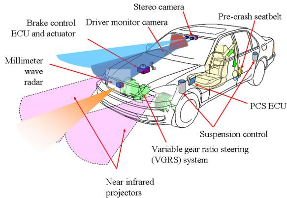
Figure 4. Configuration of PCS system with pedestrian collision avoidance assist.
