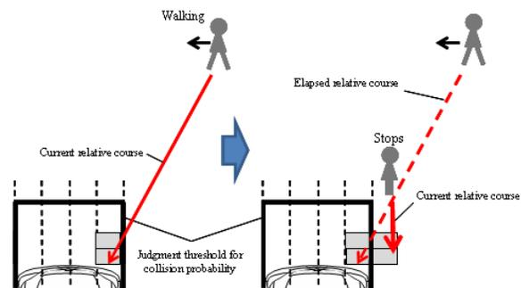
Figure 18. Collision probability distribution in false positive scenario.
