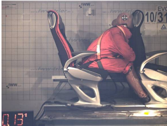
Figure 26: Dynamic test of a coach seat bench with 2 belted dummies according to ECE-R 80
