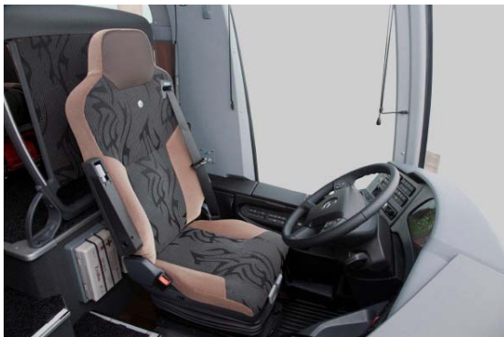
Figure 22: Coach driver seat fitted with 3-point-belt
