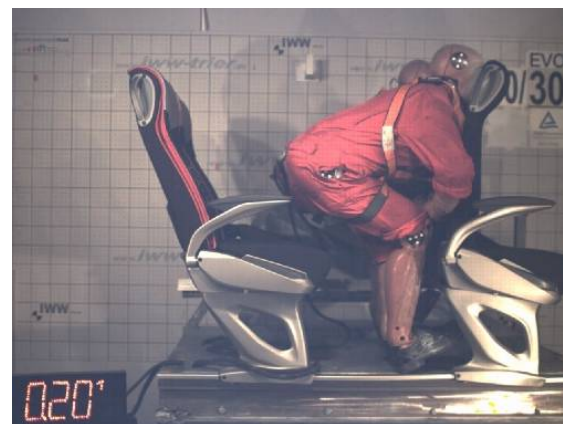
Figure 25. Dynamic test of a coach seat bench according to ECE-R 80 with 2 dummies unbelted impacting the back rest of the tested seats in front
