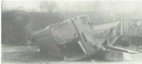
Figure 13. Rollover test on a Mercedes-Benz O 303 in accordance with ECE-R 66 conducted in 1987
