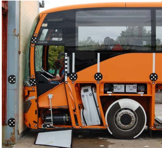
Figure 18: Coach Setra 515 HD after a full-frontal impact with a stationary rigid barrier at 25 km/h
