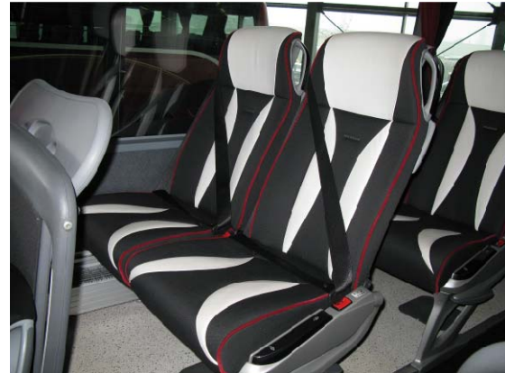
Figure 23: Coach passenger seats fitted with 3-point belts
