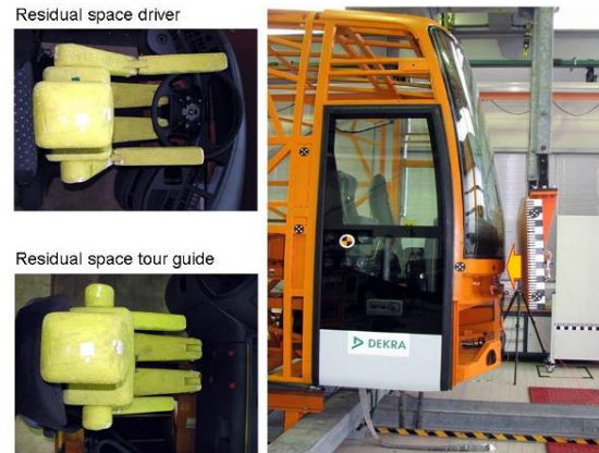
Figure 20: Mercedes-Benz Travego after frontal pendulum-impact test
