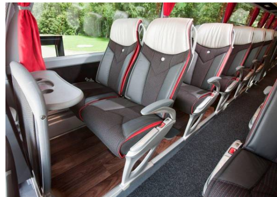
Figure 24: Coach passenger seats fitted with 2-point lap belts
