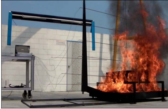
Figure 8. Fire resistance test scene according to draft of ECE R-100 in Outside
