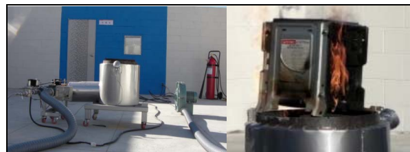
Figure1. Fire resistance test equipment and test scene according to current KMVSS test procedure
