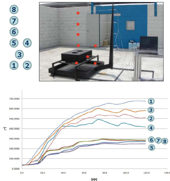
Figure 9. Flame temperature at each point
