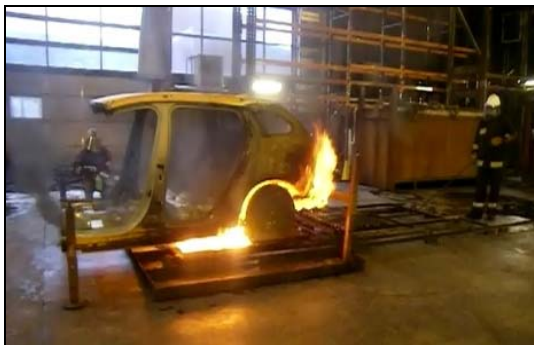
Figure 6. Fire resistance test scene according to the draft of ECE R-100(vehicle based)
