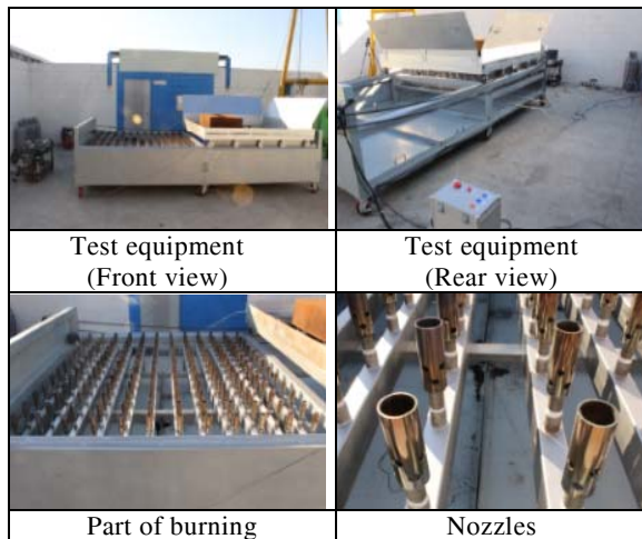
Figure 12. Fire resistance test equipment according to the draft amendment of KMVSS test procedure
