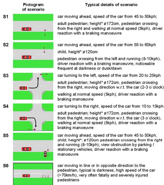
Figure 4. Scenarios for testing of pedestrian detection systems based on GDV accident data [Niewöhner, 2011].
