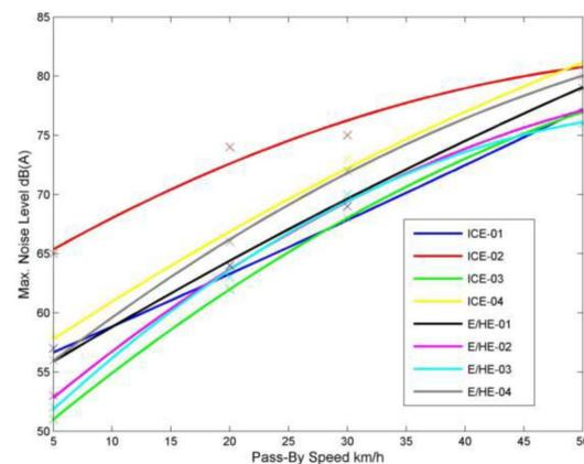
Figure 10. Maximum noise levels for steady-speed pass-by measurements [Morgan, 2011].
