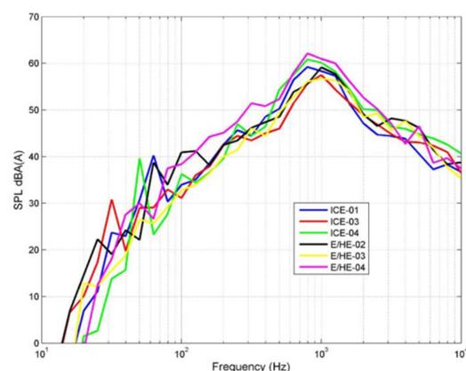
Figure 11. One third octave spectra corresponding to maximum noise level at a pass-speed of 20 km/h [Morgan, 2011].
