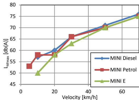
Figure 8. Sound level for different speeds.
