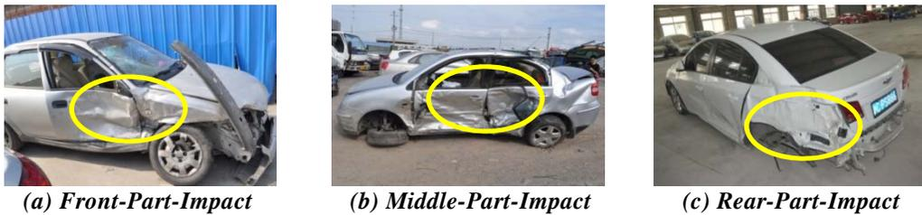
**Figure 3 classification of side impacted parts**
