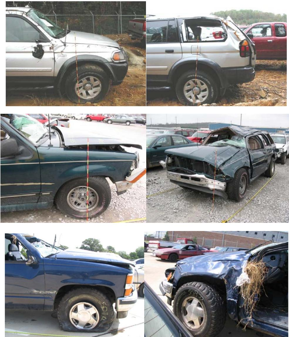
*Figure 2. Examples of vehicle panels with minor damage (left) versus major damage (right).*
