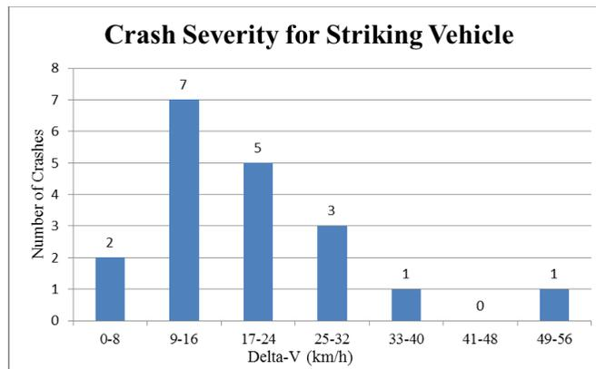
**Figure 8. EDR-Captured Crash Severity for Striking Vehicle.**
