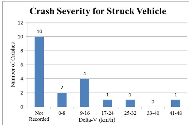
**Figure 7. EDR-Captured Crash Severity for Struck Vehicle.**
