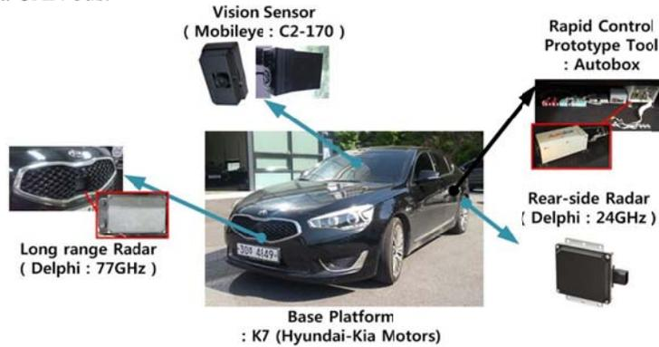
**Fig. 6 Test vehicle configuration**
