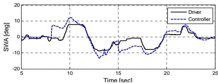
*(b) Comparison of the steering angle between the driver and the controller*
