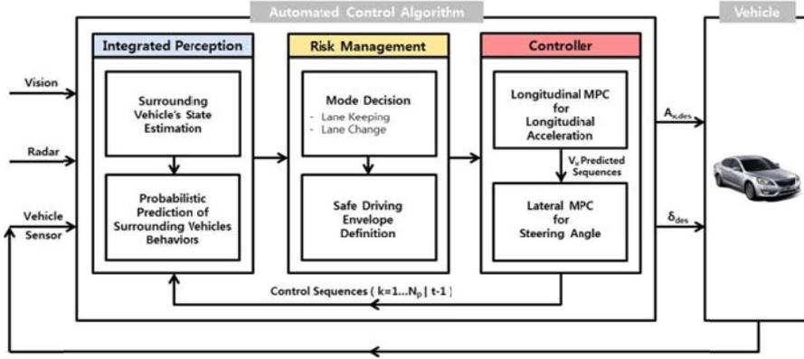
Fig. 1 Overall architecture of the proposed automated driving control algorithm
