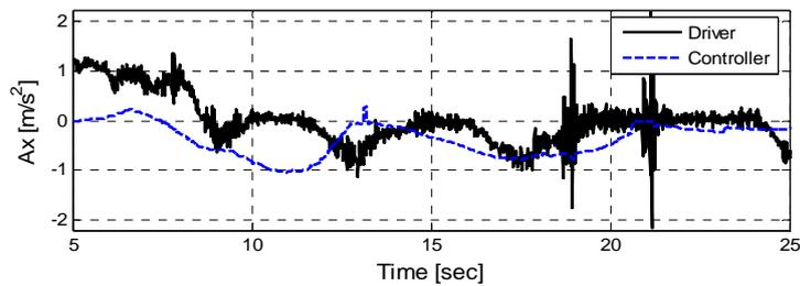
*(c) Comparison of the longitudinal acceleration between the driver and the controller*
