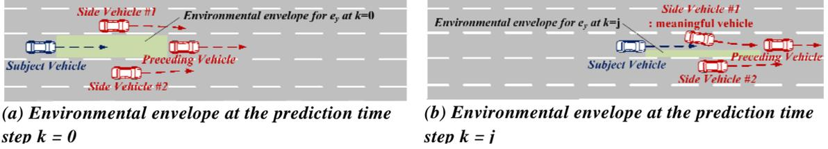
**Fig. 5 Determination of the target vehicle for the longitudinal acceleration control in a lane keeping mode**
