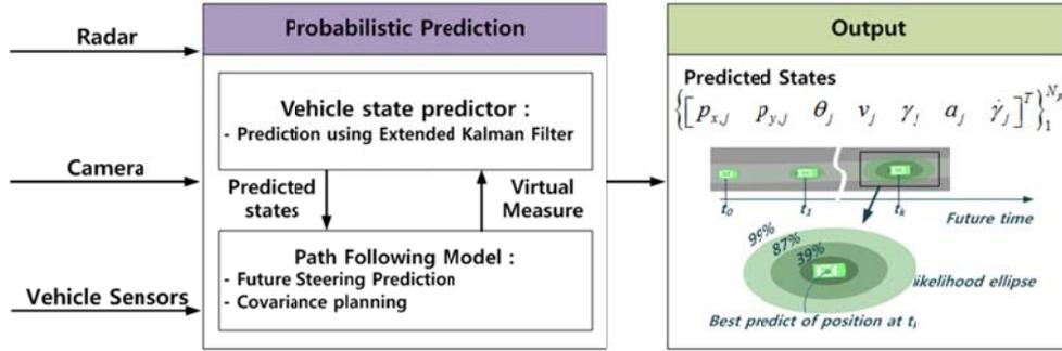
Fig. 3 Overall architecture of probabilistic prediction of surrounding vehicle's behavior
