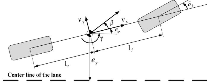
**Fig. 2 Diagram of lateral dynamics model**
