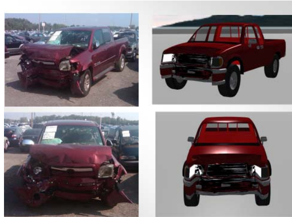
Figure 5. Images of a vehicle with frontal damage and the resulting models using FARO Blitz and FARO 360 HD software.
