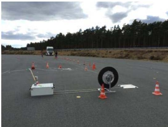
**Figure 3: Dummy propulsion system**
