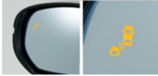
Figure 3. BSW indication method used (USNCAP target).
