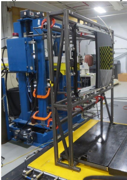
Figure 8. Sunroof module attached to custom-made frame at same locations as vehicle roof.
