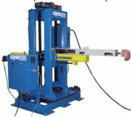
Figure 10. Ejection guided impactor with 18 kg featureless headform.
