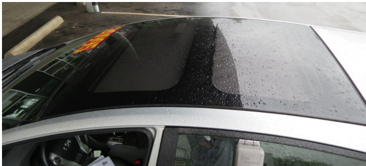
Figure 5. Toyota Prius V large polycarbonate sunroof with two daylight openings.
