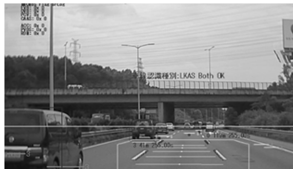
Figure A. Image of the advanced safety system recognizes the white line on the road
