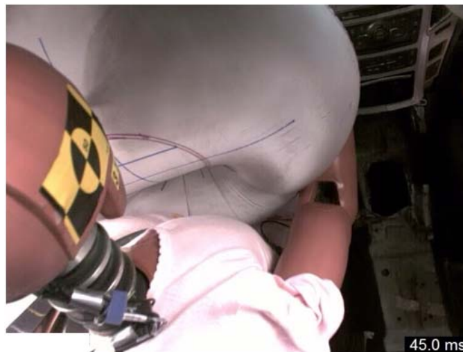
Figure 5. Interaction between asymmetric DAB and ATD chest
