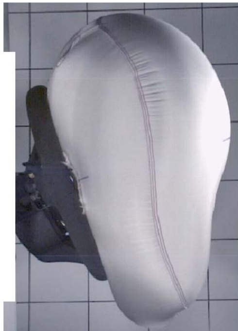
Figure 4. Smiley (asymmetric) DAB which was proposed by supplier
