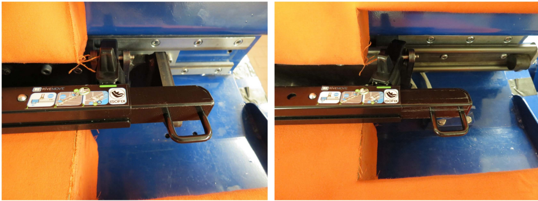
Figure 15. Resulting deformation in the RiveMove device (right) after one of the side impact tests
