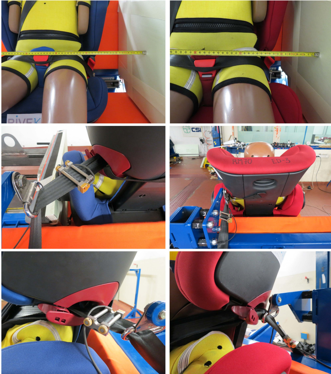
Figure 5. Positioning of the dummy mid-plane at 350mm from the door panel (left), according to ECE R129 specifications for the baseline tests. Displacement aside of the dummy mid-plane closer to the door panel in the CRS+ISOFIX accessory configuration, regulation set at 280mm (right)
