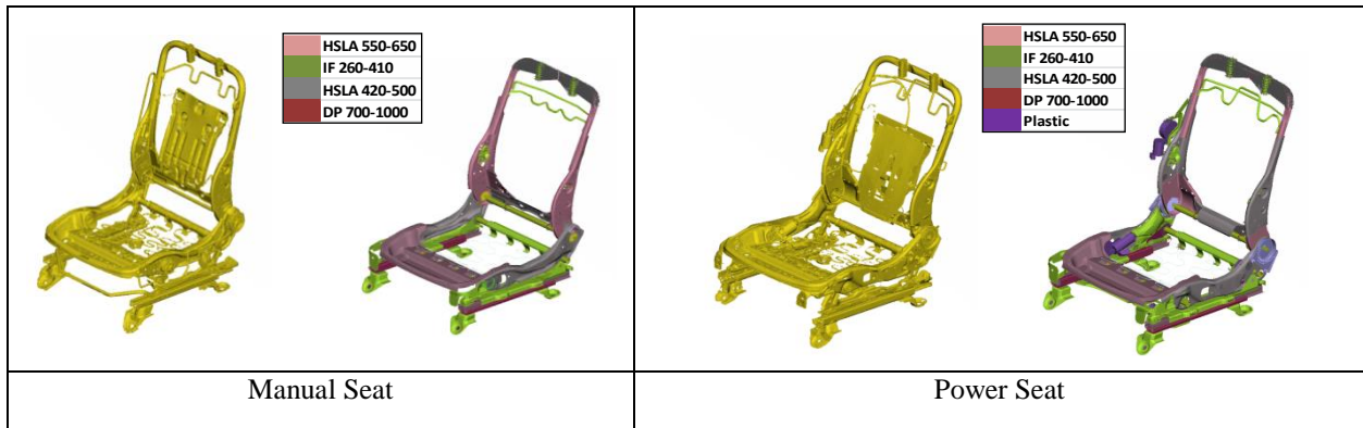
Figure 1. Scanned seat and FEA model of Manual and Power seat
