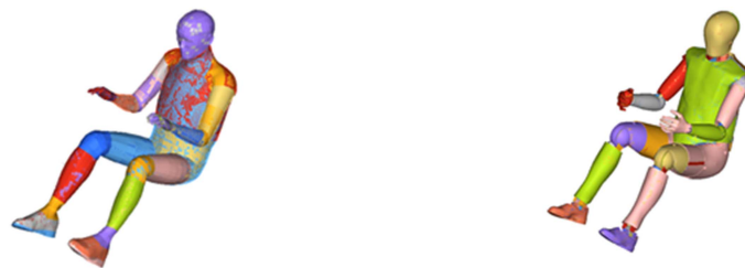
(a) Elderly occupant full body FE model (b) THOR-50th Metric FE model Version 1.4.1
