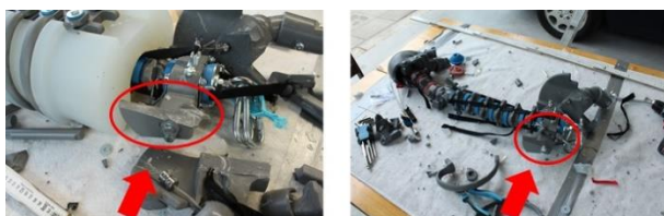
Figure 26. Fracture of the ilium next to the sacroiliac joint of the biofidelic dummy (Left: Crash test wh18.25; Right: Crash test wh18.27; Red circle: Location of fracture; Red arrow: Impact direction).
