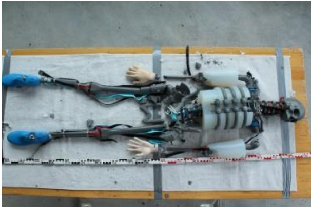
Figure 20. Overview of the "autopsy" of the biofidelic dummy used in crash test wh18.25.
