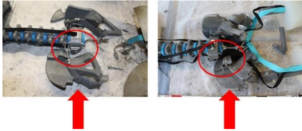
Figure 24. Fracture of the right sacroiliac joint of the biofidelic dummy (Left: Crash test wh18.24; Right: Crash test wh18.26; Red circle: Location of fracture; Red arrow: Impact direction).
