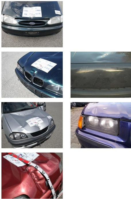
Figure 8. Vehicle damages Žilina dummy vs. pedestrian. Top left: wh08.27; Upper left: wh08.28; Lower left: wh08.29; Bottom left: wh10.12; Top right: accident 1; Bottom right: accident 2.
