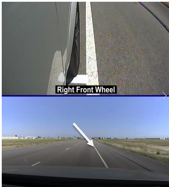
Figure 4. Point of maximum lateral deviation observed during a right-side approach test performed with the Volvo XC90 and a 0.7 m/s lateral velocity
