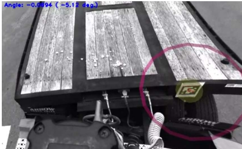
Figure 9. Example of Output from AprilTags
