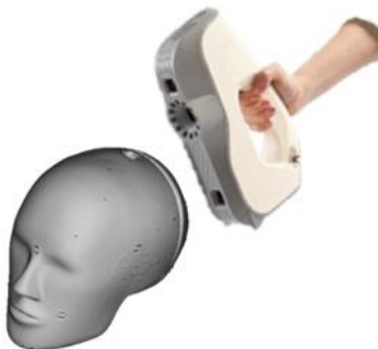
Figure 4. Head dummy to 3D mesh performed with a scanner.
