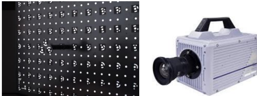
Figure 3. Calibration panel and high-speed camera with exchangeable lenses.
