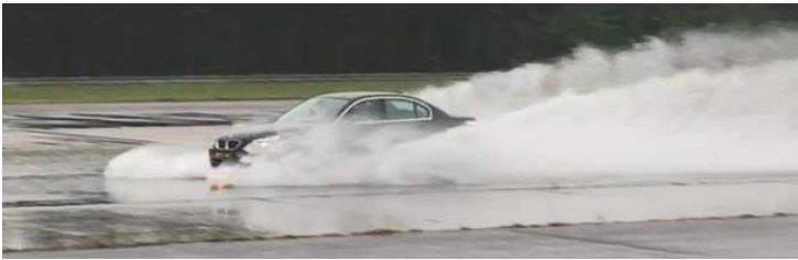
Figure 13. Hydroplaning assistance vehicle test at the “Contidrom” proving ground with front wheels floating. The vehicle is controllable by rear wheel brake torque vectoring
