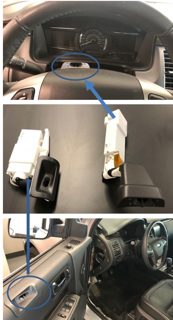
Figure 4. DADSS Breath-based sensors; Steering column (top) and driver-side door (bottom)
