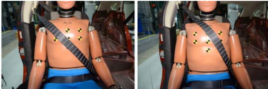
Figure 7. Belt Routing 50th Male Dummy D-ring Down (Left) and D-ring Up (Right) – Dodge Caliber
