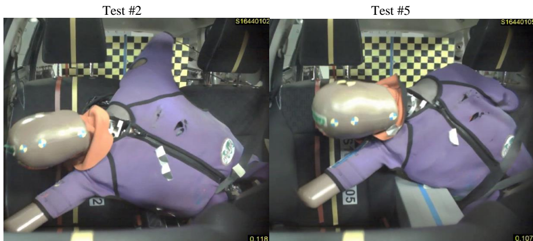
Figure 17: With and without centre console max excursion
