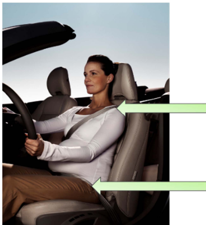
Figure 3. Example of interacting with strong body parts. The three point seat belt should be positioned over the pelvis and across the chest and shoulder.
