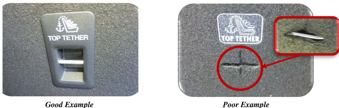
Figure 8. Examples of good and poor top tether execution
