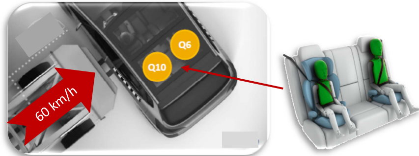
Figure 22. Side impact mobile deformable barrier (MDB) test
