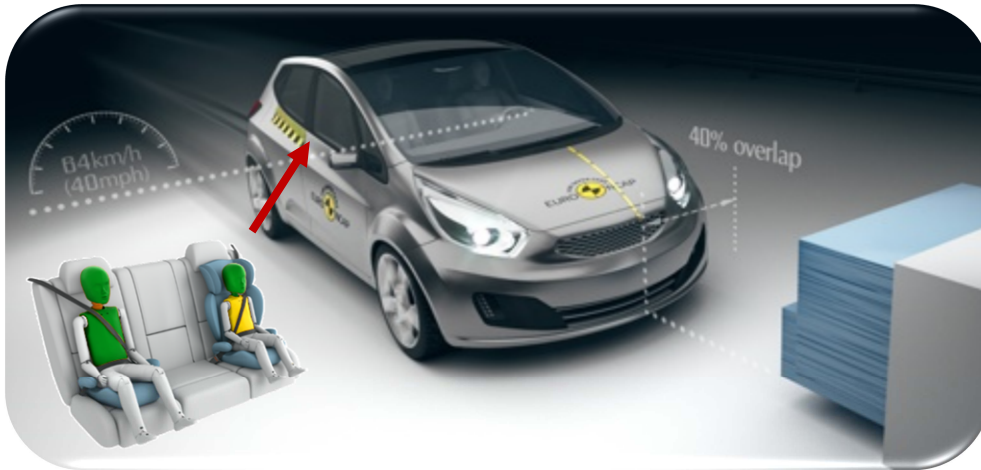
Figure 2. Frontal impact offset deformable barrier (ODB) test [5]
