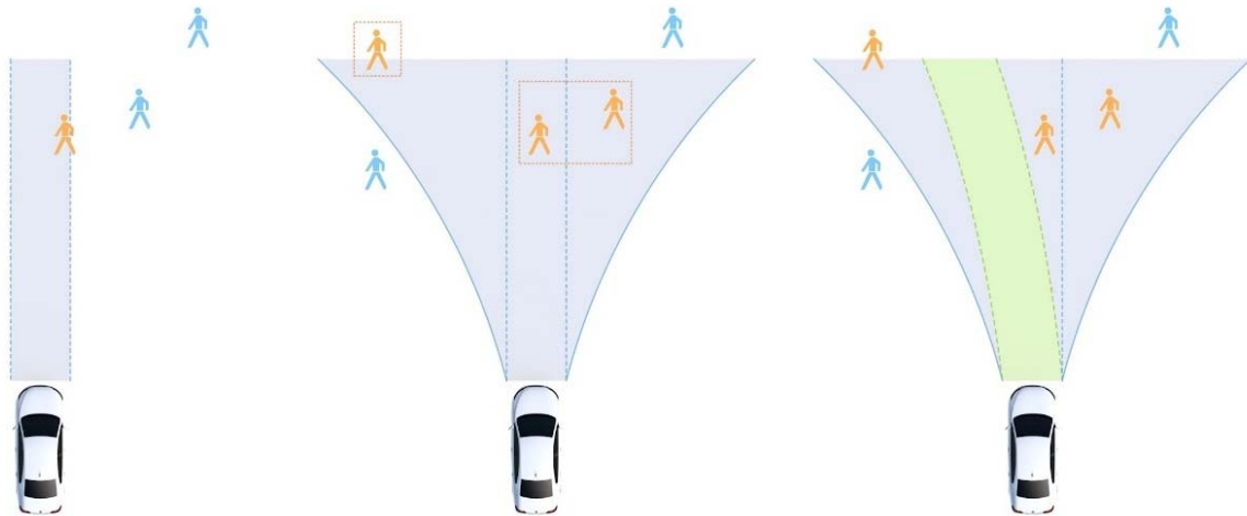
Figure 4. The steps for identification of a collision-free vehicle path (for simplicity the motion of pedestrians is not represented). From left to right: a pedestrian is identified in the vehicle's path; other pedestrians are identified in the accessible region; a collision-avoidance path between groups of pedestrians is determined.
