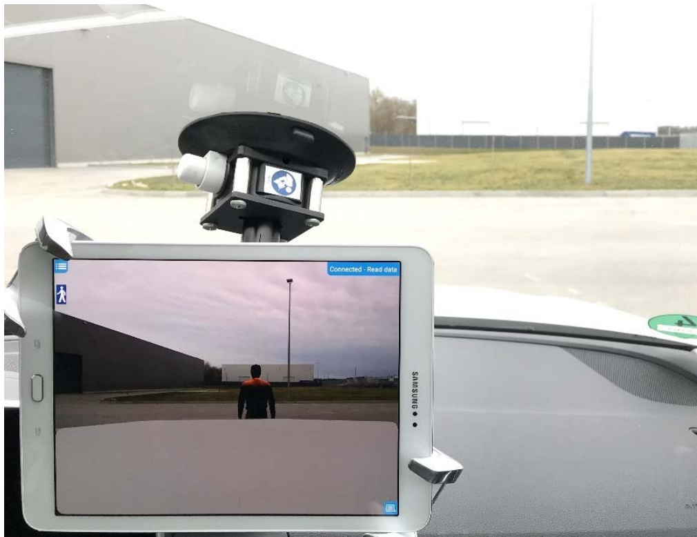
Figure 5. Inside IAV's Vehicle-in-the-Loop: the test scenario is visualized in a display showing the (real) environment and the (virtual) pedestrians.
