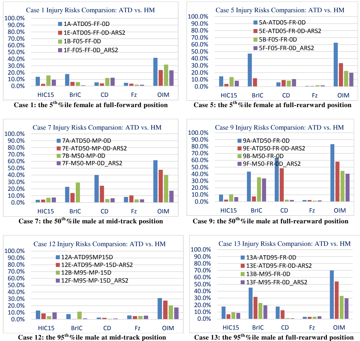
Figure 4. Comparison of the HM predicted Occupant Injury Measures with the ATD estimated ones for the six load cases
