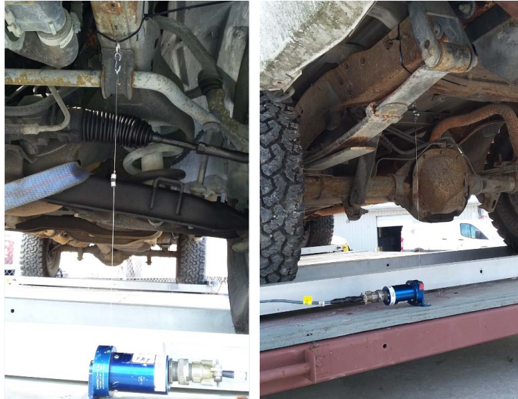
Figure 3 Front (left) and rear (right) string potentiometer placement
