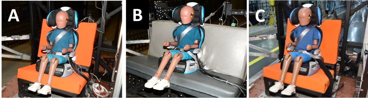
Figure 1. The Hybrid III 6-year-old installed in a high-back booster seat on (A) the proposed FMVSS bench + accel sled, (B) the CMVSS bench + acceleration sled, and (C) the proposed FMVSS bench + deceleration sled.
