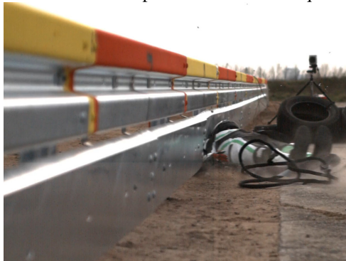
Figure 3: Impact according CEN/TS 1317-8:2012 (source: DEKRA)
