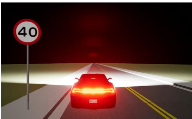
Figure 9. Detection of speed sign during the night by ego vehicle.
