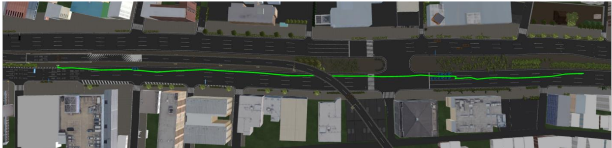
Figure 7. Riding trajectory on the road from reconstruction simulation
