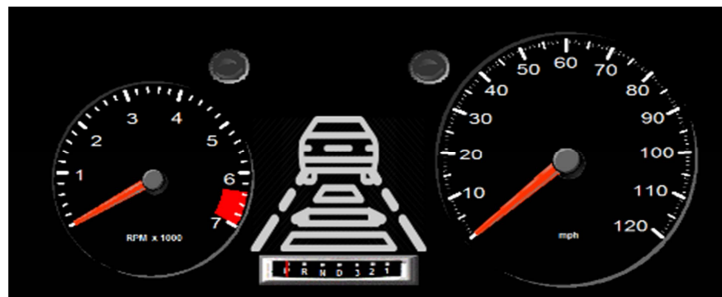
Figure 1. Instrument panel with ADS information available in the center.
