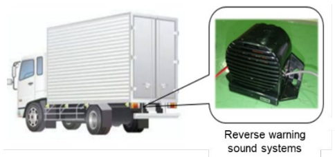
Figure 3. Installation example of reverse warning sound systems
