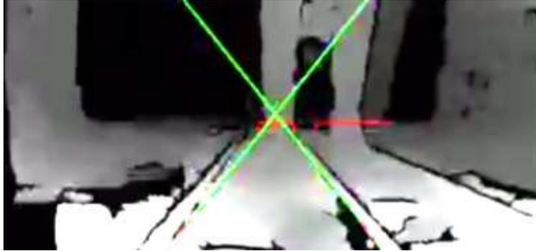
**Figure 5.** Depth map algorithm detecting a complete roadblock as objects exist in both lanes
