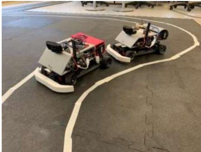
**Figure 1.** The two 1/10 scale RC cars with hardware modifications featuring the original cameras
