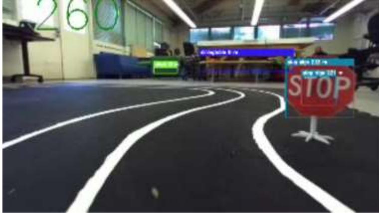
**Figure 3.** Fast YOLO neural network identifying multiple objects including a stop sign
