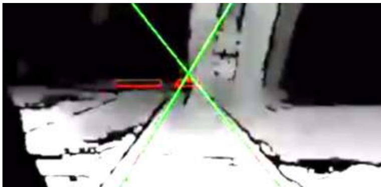
**Figure 4.** Depth map algorithm identifying an object in the current lane and the left lane available for a lane change
