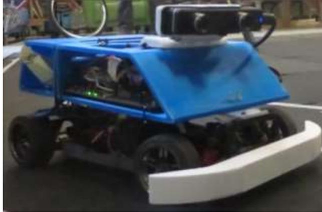
**Figure 2.** One 1/10 scale RC car with hardware modifications featuring a stereoscopic camera
