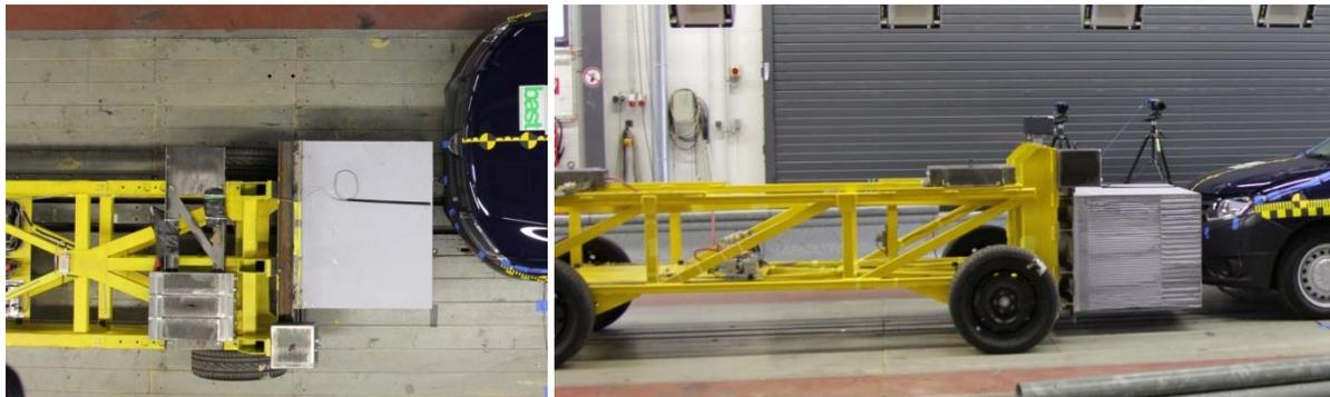
**Figure 1 Crash trolley used of the test with mobile barrier specified in [7] using the PDB v8.0 XT**
