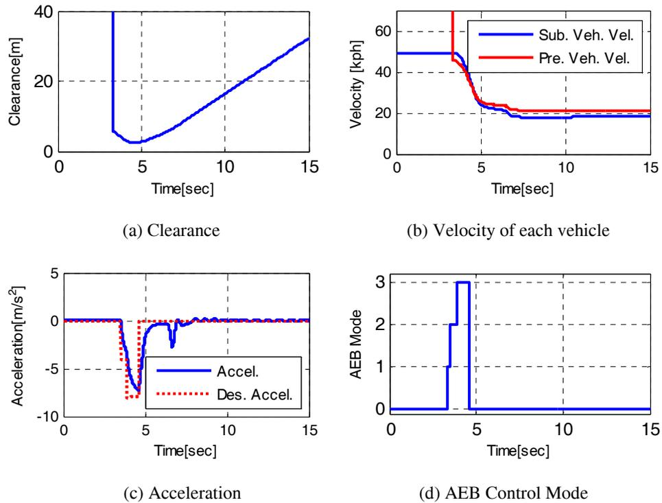
**Figure 2.** Simulation result of AEB system in preceding cut-in with decelerating vehicle scenario.
