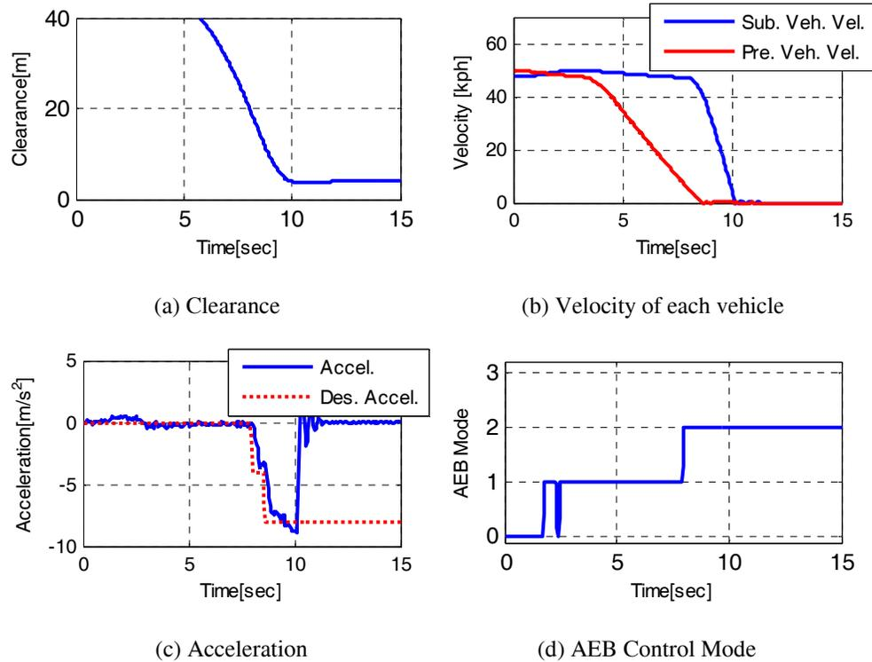
*Figure 3. Test result of AEB system in preceding decelerating vehicle scenario.*
